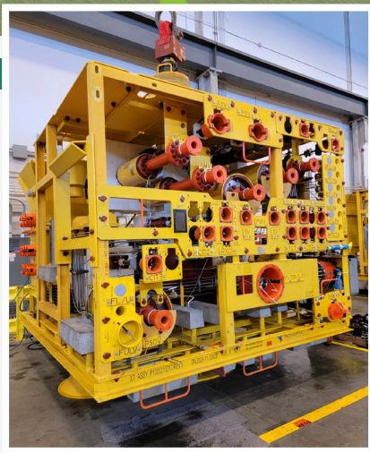
Stampede subsea production well tree
