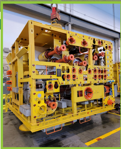
Stampede Subsea Production Well Tree
